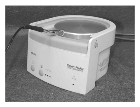
Figure 7.1: Location of test point on heater plate
