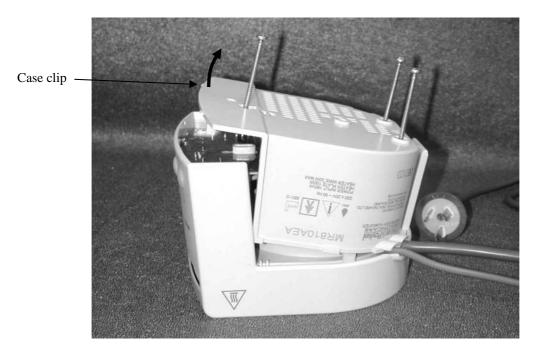
Figure 6.1: Removing the case bottom
